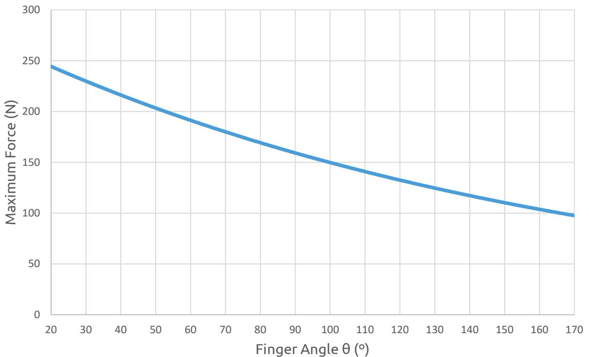
Graph plotted using measurements with 1 A current, silicone fingertips and a metal workpiece.
