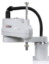
**SCARA** (Selective Compliance Assembly Robot Arm) industrial robots are rigid in the Z-axis and compliant in the XY-axes. They excel at:
